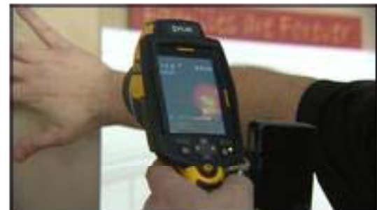
Home energy inspector Mitch Richardson used a thermal camera to detect where the heat was going in Shelly Bouvang's house.
